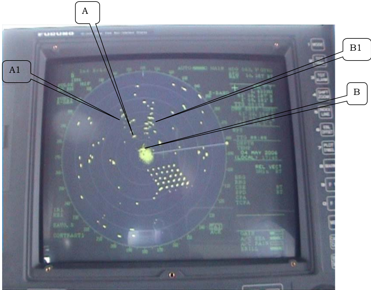
Figure 4.14: Examples of Incomplete External Mirror Images
