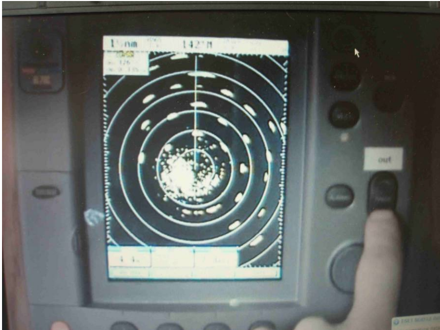
Figure 5.6: Sailing yacht radar, ship's head up display with yacht heading south east
