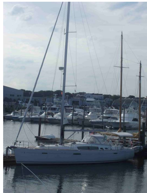
Figure 5.7: Sailing yacht: Note radar antenna (enclosed) at almost half height of mast just above lower cross-trees.
