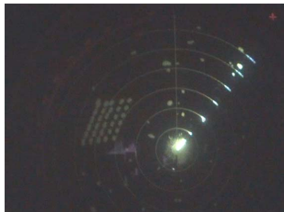
Figure 4.17: Master ordered the cargo crane jib to be re-stowed and effect disappeared
