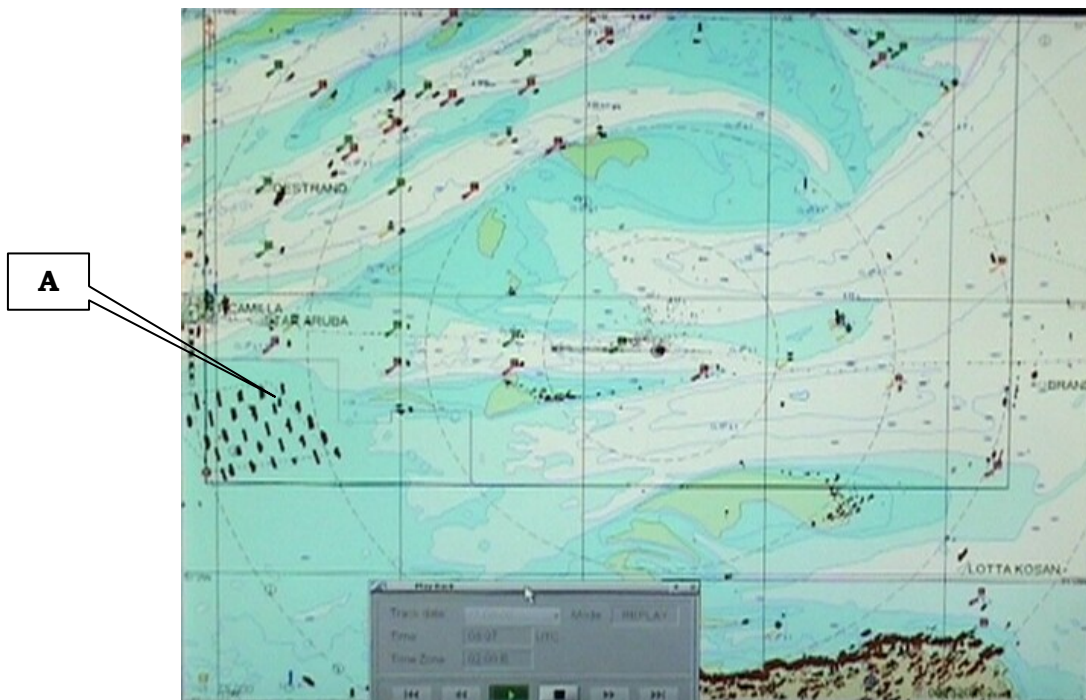
Figure 5.2 (above): Image from a tanker with electronic chart display overlaid with radar
